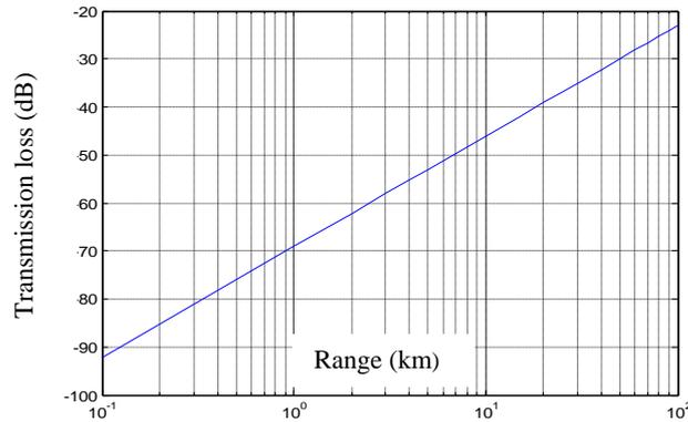
Fig.6 Typical transmission loss curve of band limited signal
