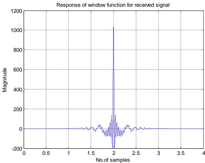
Fig. 19 Envelope of matched filter output passed through window
