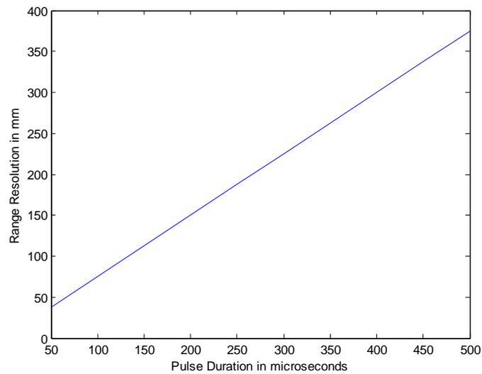
Fig. 10 Variation of range resolution for various pulse durations for fixed frequency sonar
