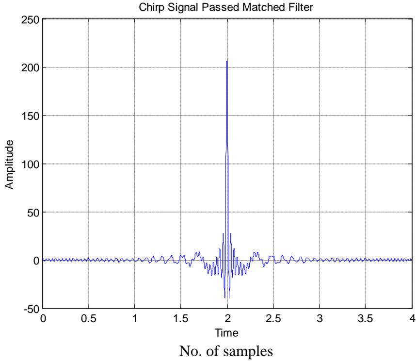
Fig. 19 Response of matched filter for received signal
