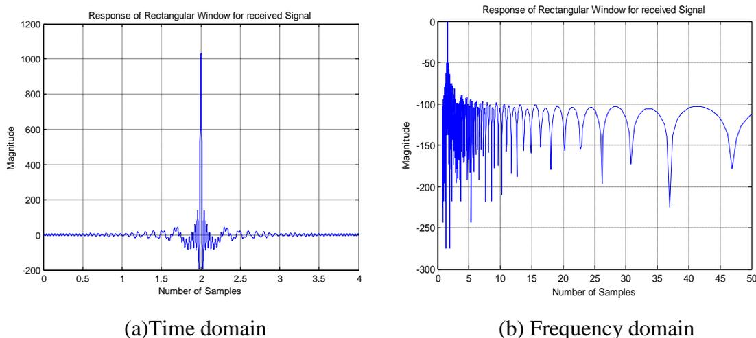
Fig. 20 Magnitude response of received signal after rectangular window
