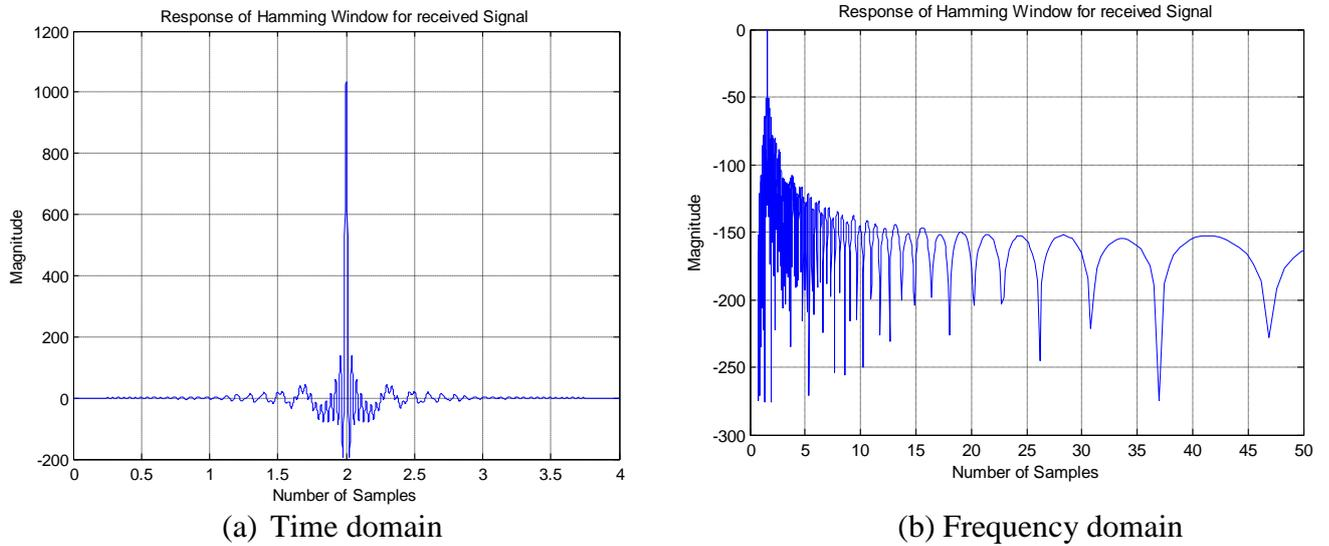
Fig. 22 Magnitude response of received signal after hamming window
