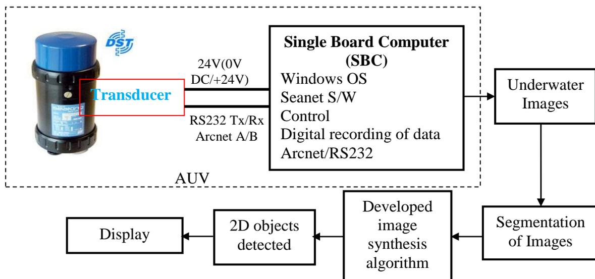
Fig. 33 Experimental setup for collecting sonar data
