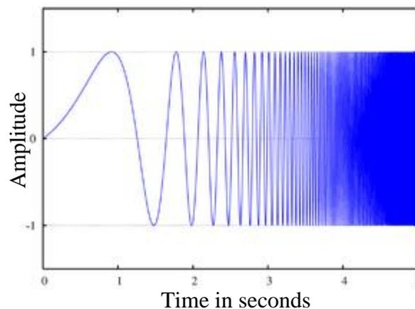
Fig.15 An exponential chirp waveform
