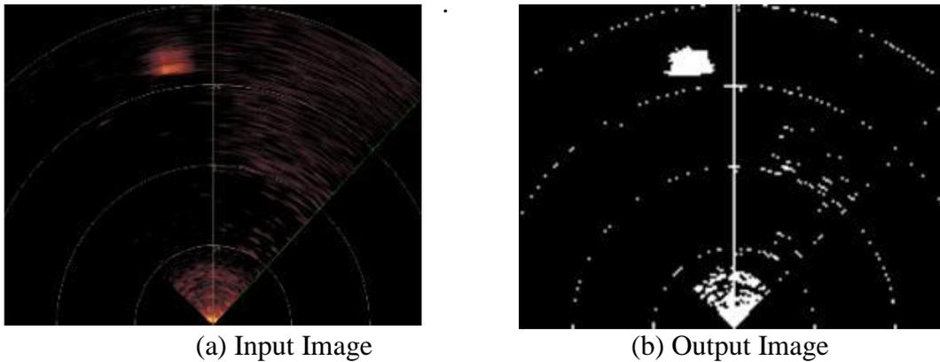
Fig. 27 Results of the Edge detection method
