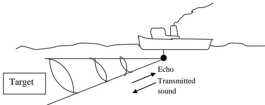
Fig. 1 Principle of operation of sonar
