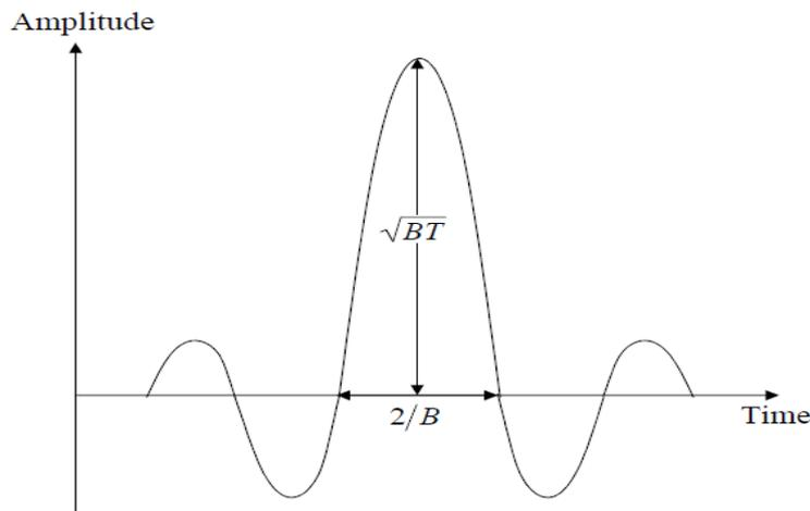
Fig. 18 Typical output from a pulse compression filter
