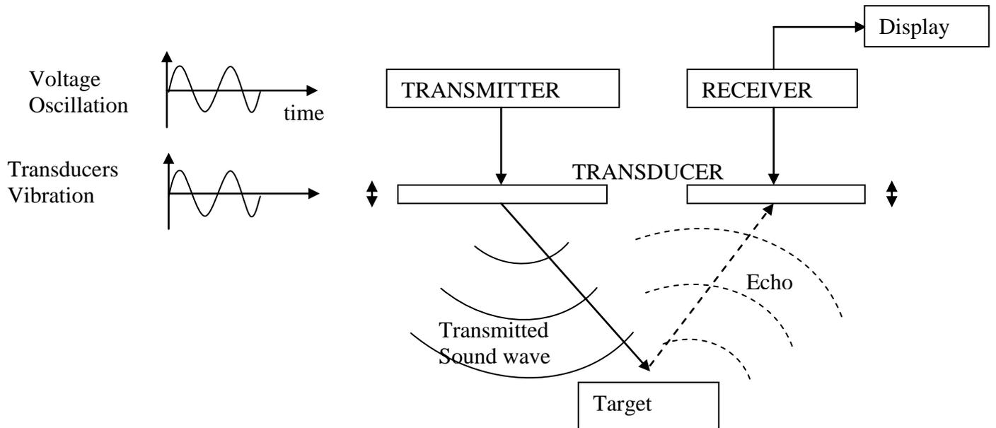
Fig. 2 Block diagram of active sonar
