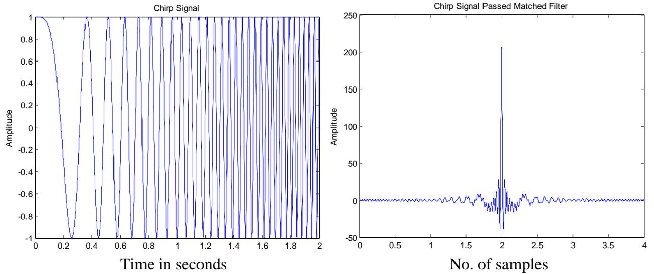
Fig. 17 b) Response of matched filter for a chirp signal
