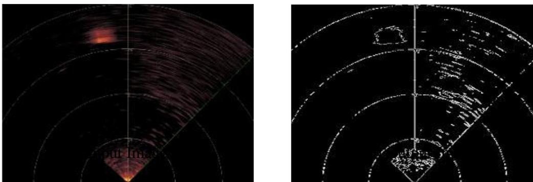
Fig. 28 Results of the Canny Edge detection method
