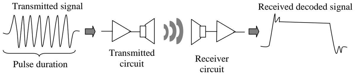
Fig. 8 Monotonic sonar acoustic signals
