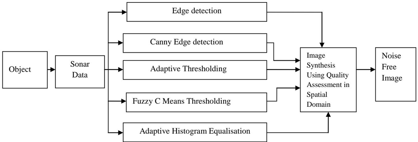
Fig. 32 Block diagram of sonar image synthesis
