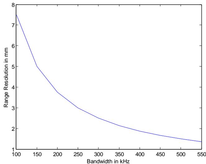
Fig. 13 Variation of range resolution for various bandwidths for chirp technology
