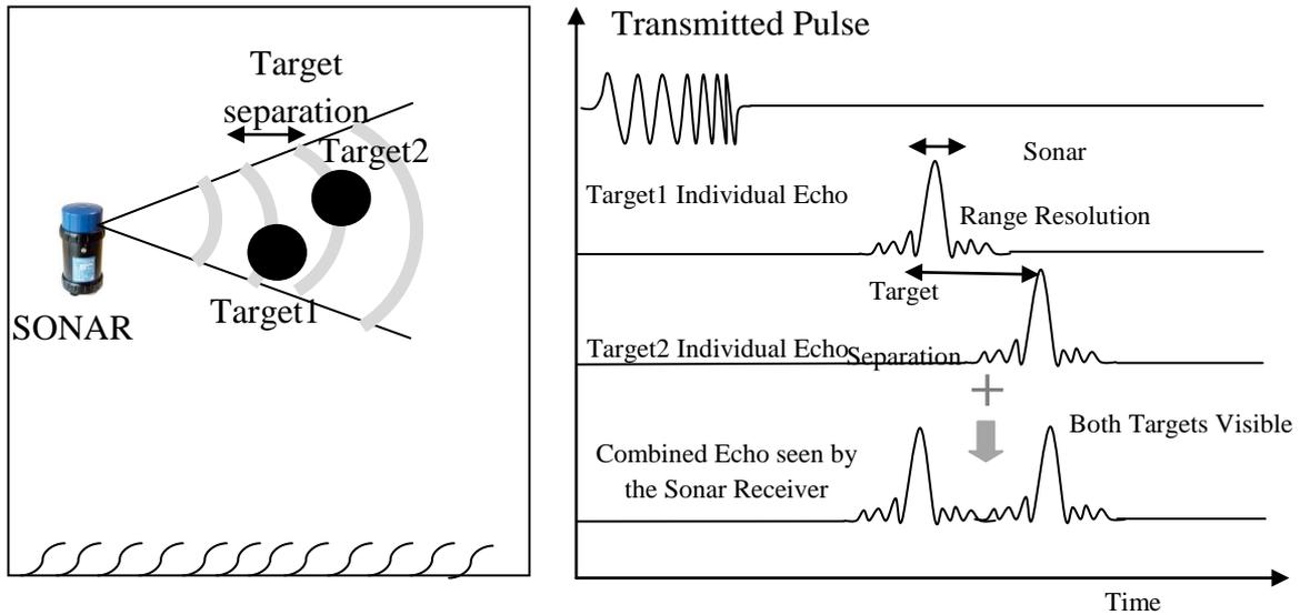
Fig. 12 Chirp sonar receiver resolution
