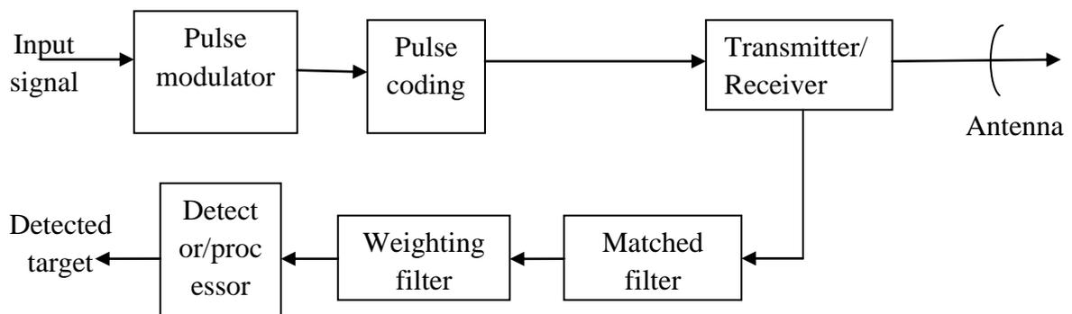
Fig. 16 Block diagram of pulse compression sonar
