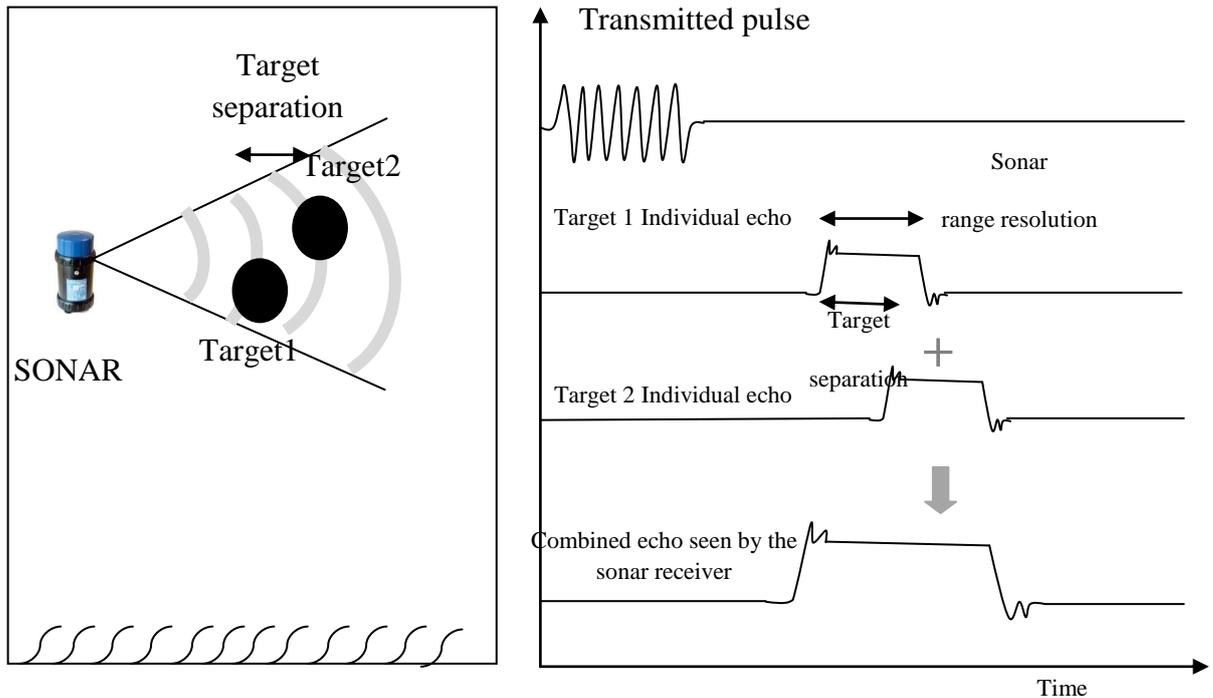
Fig. 9 Monotonic sonar receiver resolution
