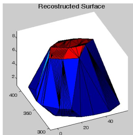
Fig. 42 Reconstruction of the object by rolling the sphere over the triangles
