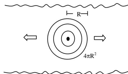
Fig. 3 Spherical spread
