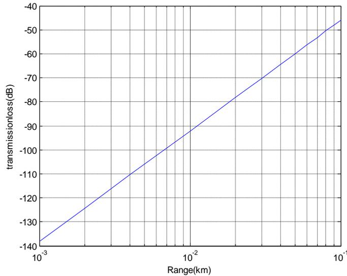
Fig. 1 Typical transmission loss curve of band limited signal
