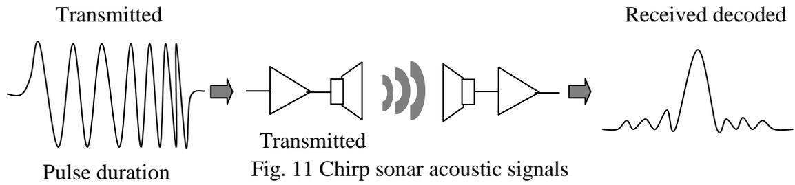
Fig. 11 Chirp sonar acoustic signals
