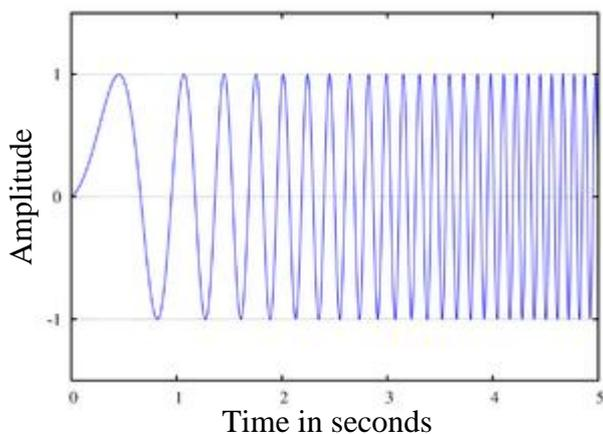
Fig. 14 A linear chirp waveform
