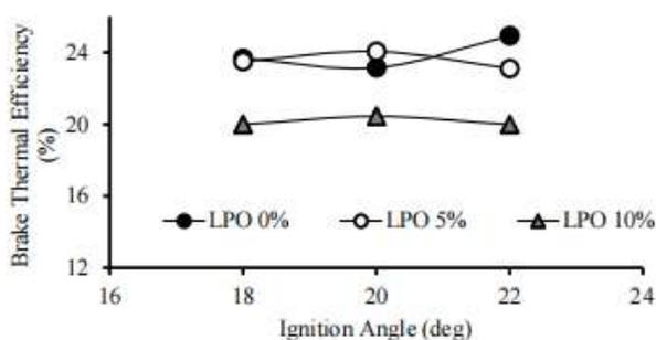
**Figure: 4.6** Variation of Brake thermal efficiency with ignition angle for different blends
