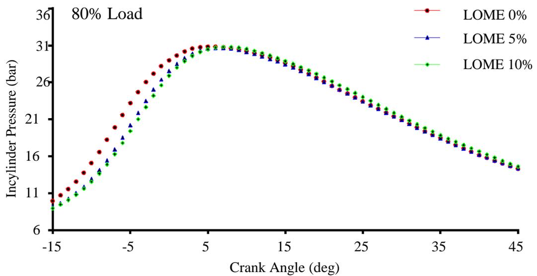
**Figure: 4.5** Variation of In-cylinder Pressure with Crank angle (deg) at 80% Load
