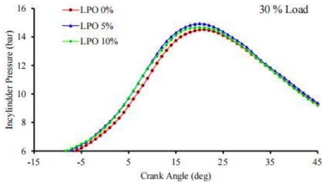
**Figure: 4.1** Variation of In-cylinder Pressure with Crank angle (deg) at 30% Load
