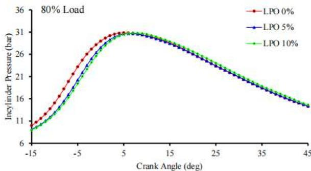
**Figure: 4.3** Variation of In-cylinder Pressure with Crank angle (deg) at 80% Load
