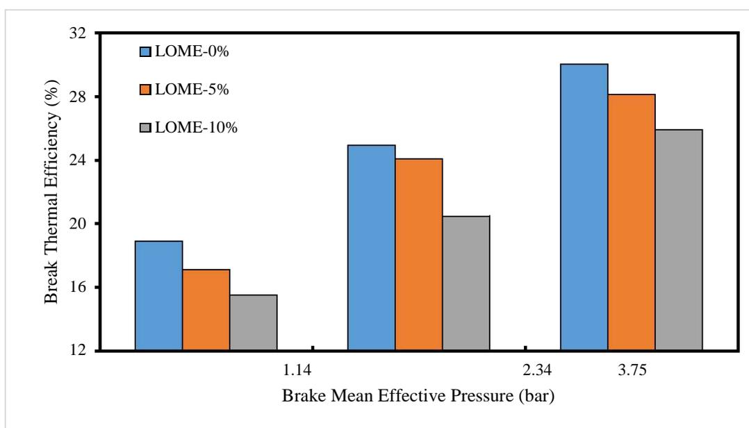
**Figure: 4.1** Variation of Brake Thermal Efficiency with Break mean effective pressure
