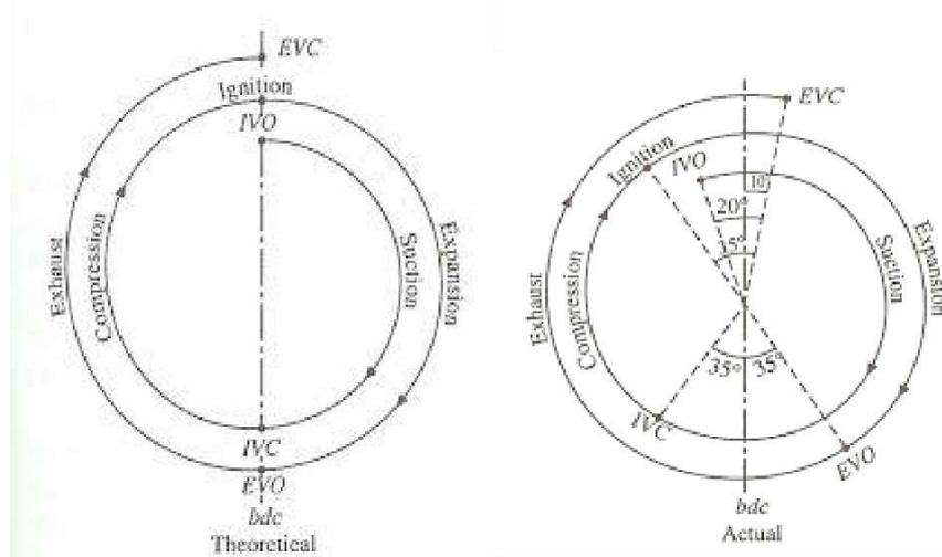
**Figure: 1.5** Valve Timing Diagrams
