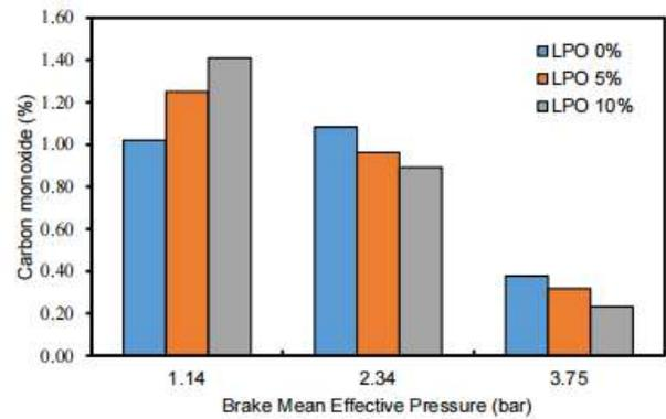
**Figure: 4.4** Variation of CO emission with different load conditions
