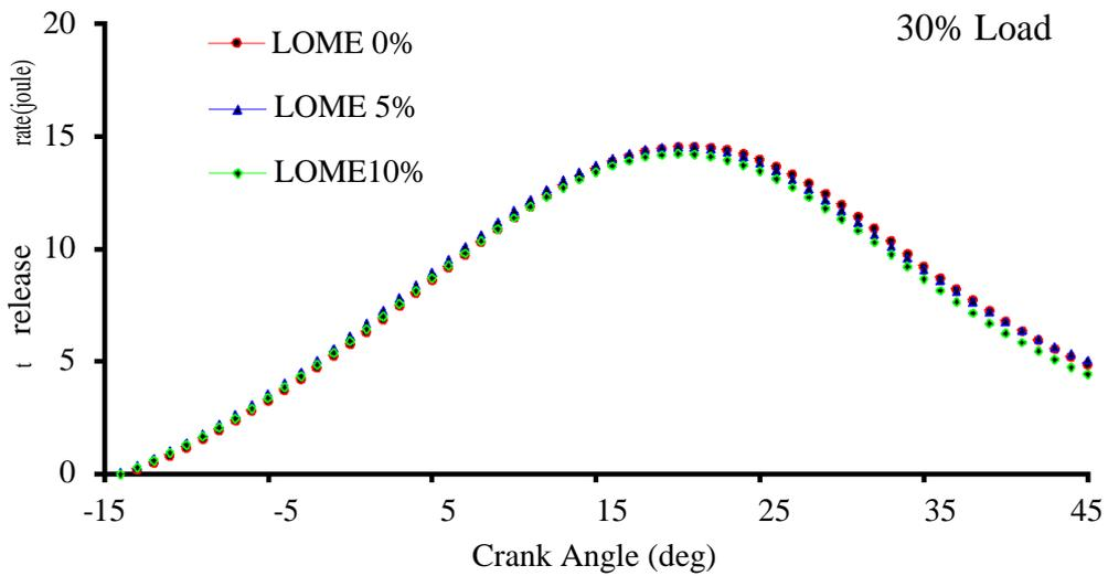
**Figure: 4.6** Variation of Heat release rate with Crank angle (deg) at 30% Load
