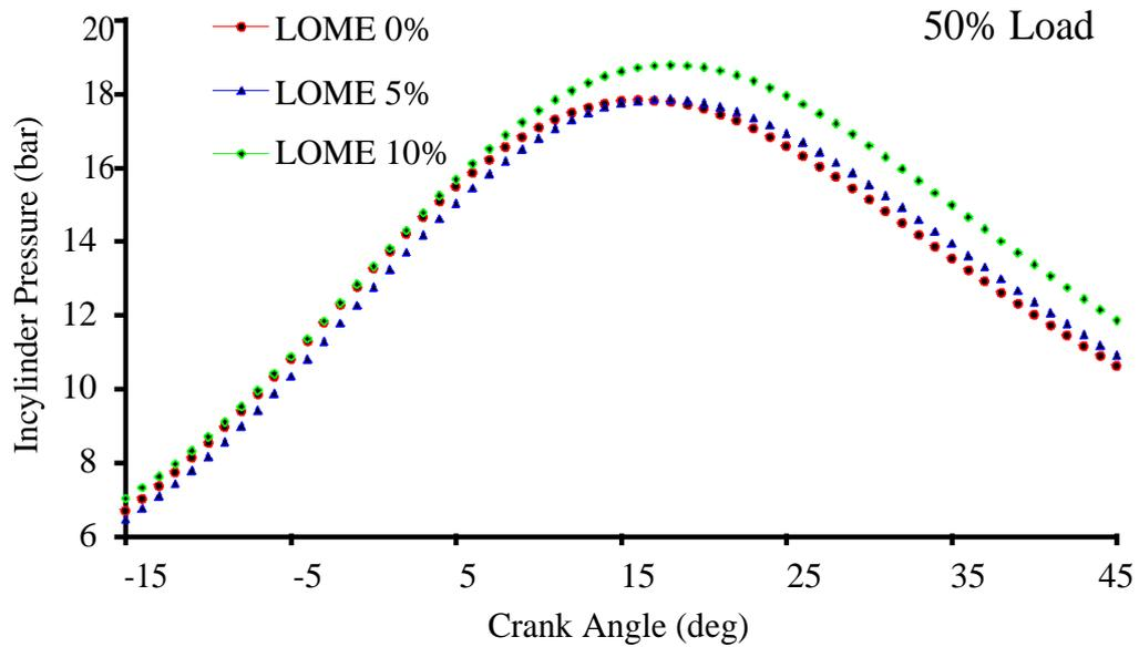
**Figure: 4.4** Variation of In-cylinder Pressure with Crank angle (deg) at 50% Load
