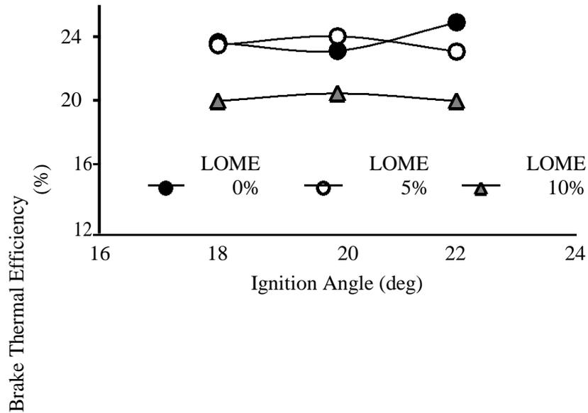
**Figure: 4.11** Variation of Break thermal efficiency with injection angle for different blends
