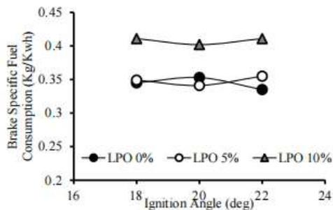
**Figure: 4.5** Variation of BSFC with ignition angle for different blends
