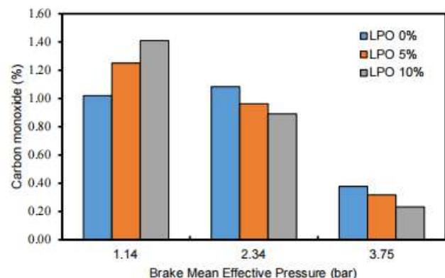
Figure 1: Variation of CO emission with different load conditions
