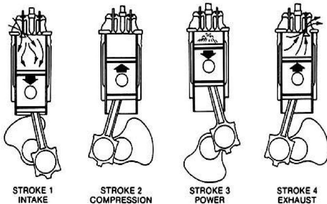
**Figure: 1.4** Working of an IC Engine
