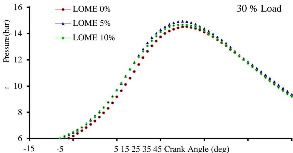
**Figure: 4.3** Variation of In-cylinder Pressure with Crank angle (deg) at 30% Load
