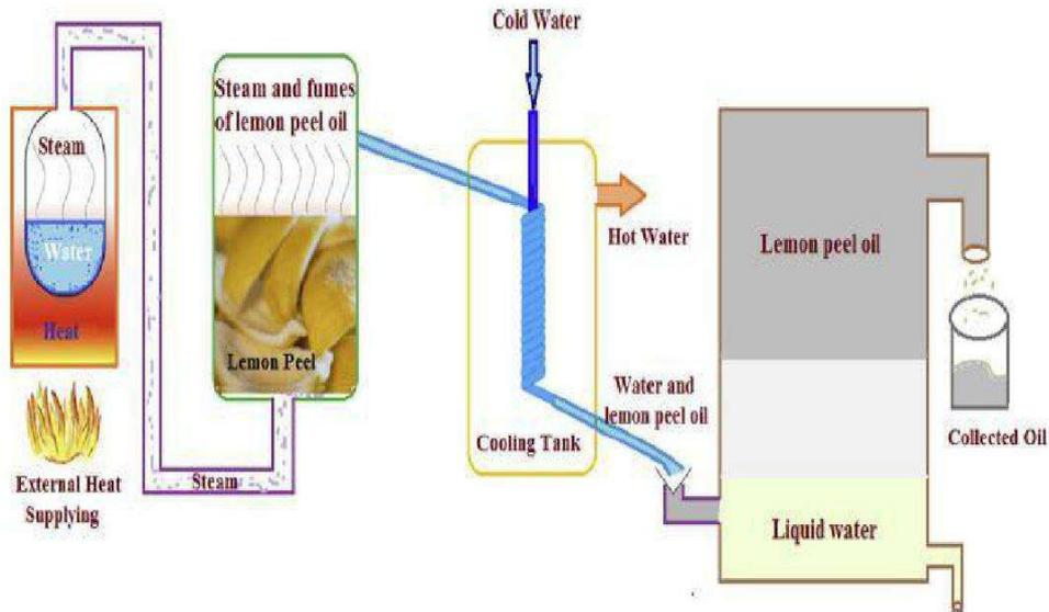
**Figure: 3.5** LOME Extraction Setup
