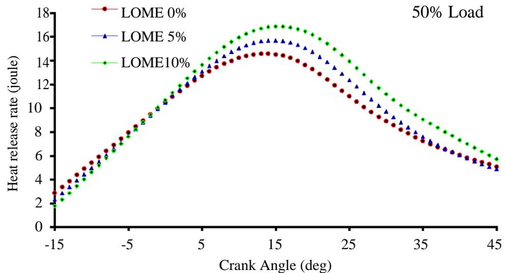
**Figure: 4.7** Variation of Heat release rate with Crank angle (deg) at 50% Load
