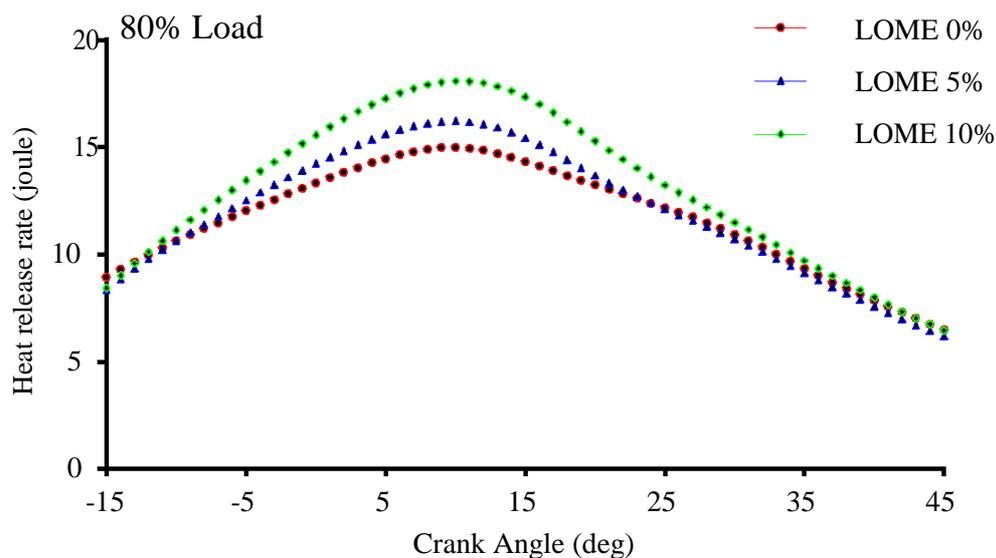
**Figure: 4.8** Variation of Heat release rate with Crank angle (deg) at 80% Load
