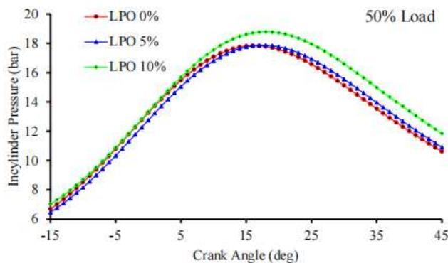
**Figure: 4.2** Variation of In-cylinder Pressure with Crank angle (deg) at 50% Load
