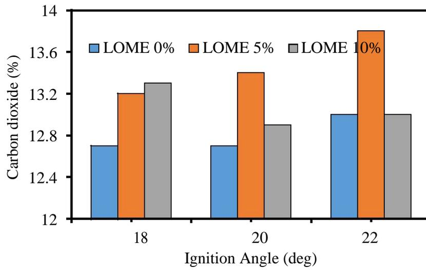
**Figure: 4.15** Variation of Carbon dioxide with ignition angle for different blends
