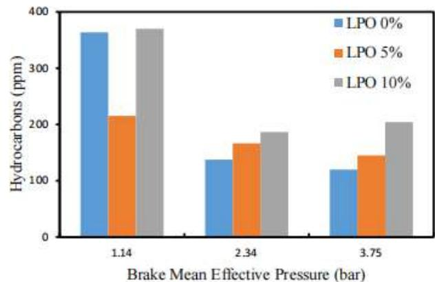
**Figure 4.4:** Variation of HC emission with different load conditions
