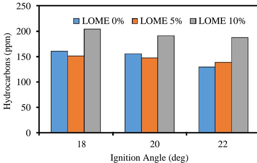
**Figure: 4.14** Variation of Hydrocarbons with ignition angle for different blends
