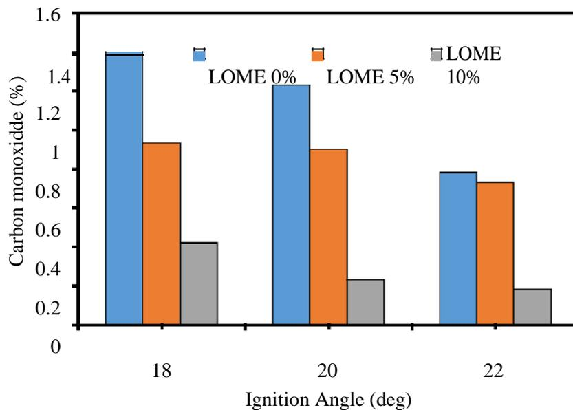
**Figure: 4.13** Variation of Carbon monoxide with ignition angle for different blends
