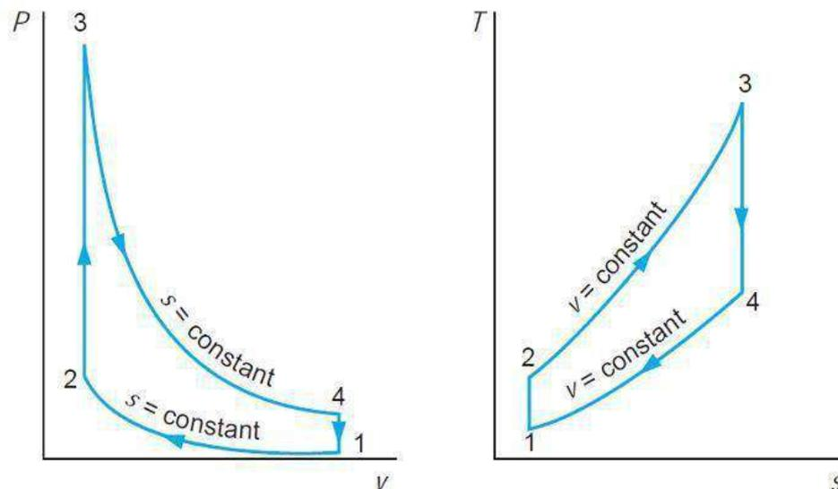
**Figure: 1.6** P-V & T-S Diagrams
