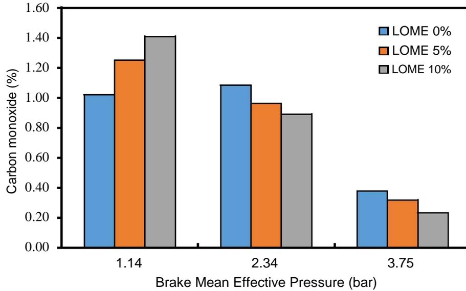
**Figure: 4.9** Variation of CO emission with different load conditions
