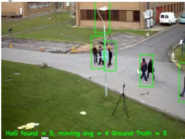
Fig. 18 Sample frame from Integer arithmetic approximation of the HOG algorithm used for pedestrian detection
