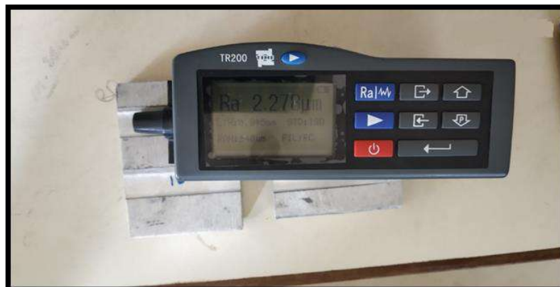
Fig 4.18: Measuring of surface roughness using Talysurf
