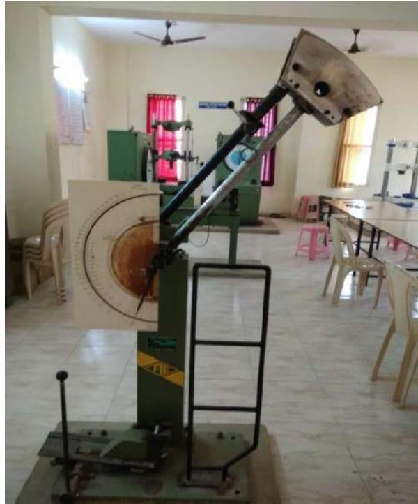
Fig.4.7 Impact testing machine (Charpy test)
